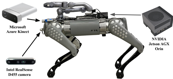
Fig. 4: The mobile manipulation platform. A 7-DOF Z1 robotic arm is mounted on top of the B1 quadrupedal robot. A forward facing Kinect sensor and RealSense camera are mounted at the front, and a Nvidia Orin onboard computer is mounted at the rear.
