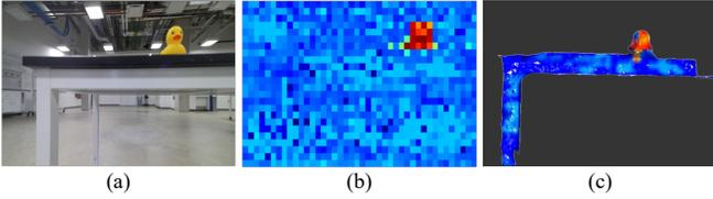
Fig. 4: **GeFF compresses and refines multi-view observations:** (a) single RGB view; (b) coarse 2D CLIP heatmap with query ‘toy duck’; (c) 3D heatmap from GeFF with clean boundary reconstructed from compressed latent representation.
